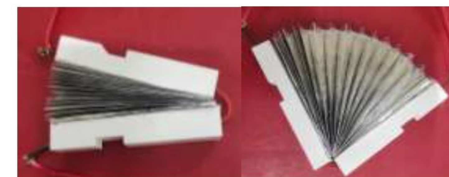
Fig 5: Closed (around 0 degree) and Opened position (90 degree) of the Light Solar Sail Prototype
