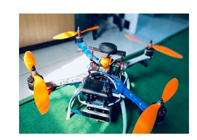
Above are some of our Quadrotors developed/ extended at the RRC, and equipped with RGB Cameras, Depth Cameras, RTK GPS, 6-DOF IMUs. The central theme is to develop systems that use low-cost low-compute sensors to perform the above stated tasks with reasonable accuracy and can run on computers on-board the vehicle.
