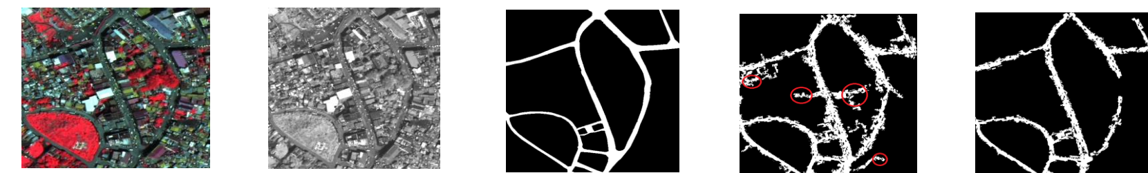
Fused Image PAN Image Road Ground truth Road extracted by ATM-R Road Extracted by ASTM-R
