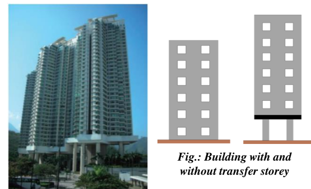
Fig.: Building with transfer storey
