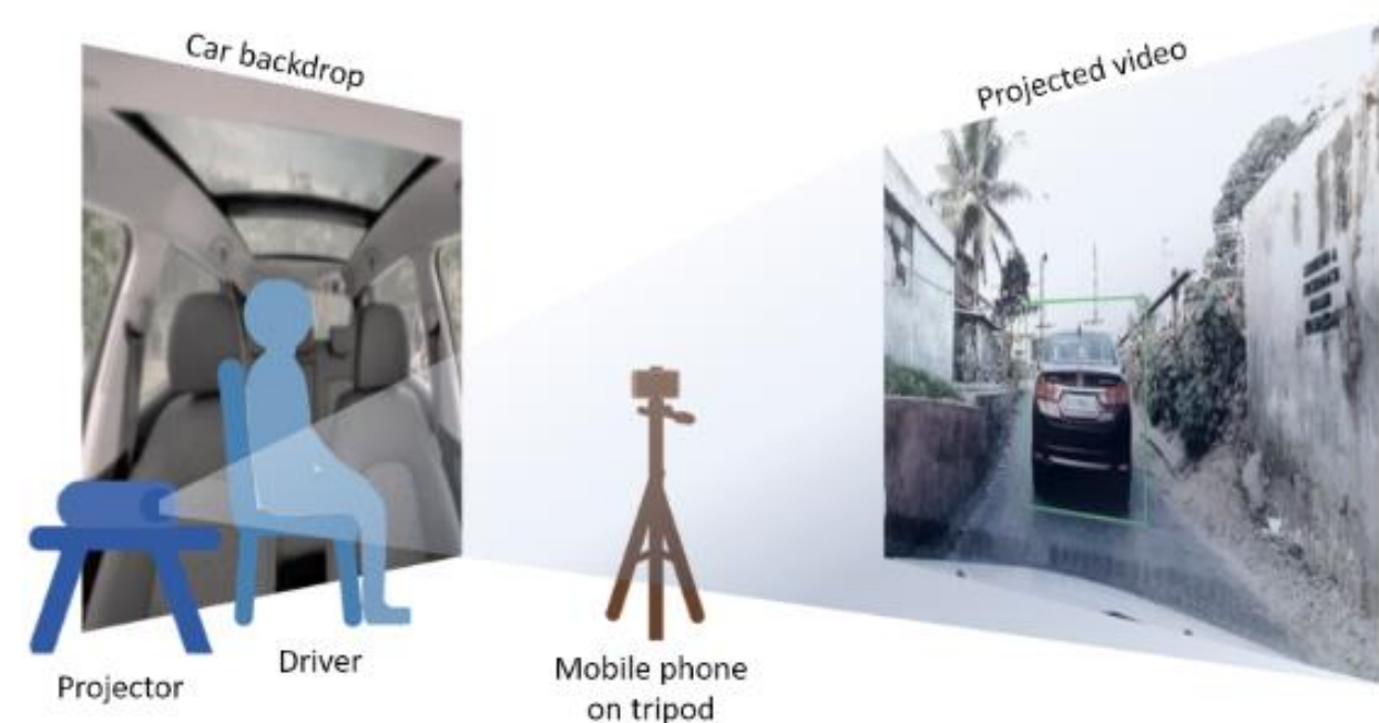
DGAZE collection lab setup
